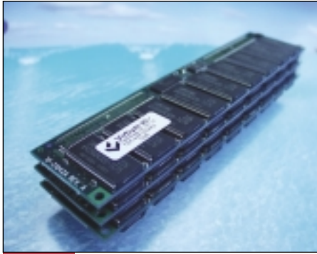
Figure 2 Virtium's CompactRAM memory module design offers staged upgrades, required functions such as error correction and registered memory module technology, significantly reduced space requirements and two to three times the memory density in a single VME or CompactPCI slot. Adding stacked components can further increase density delivering 2 to 3 Gbytes within a single frame.
